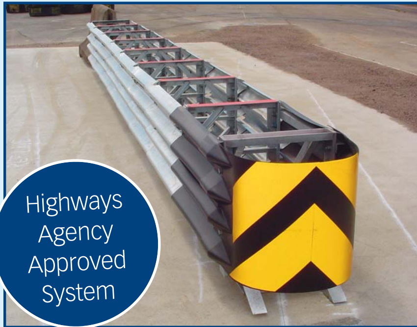
The EuroTRACC crash cushion has been successfully tested to EN 1317-3, class 110, redirective with an ASI of \leq 1,0 (class A) for all tests.
