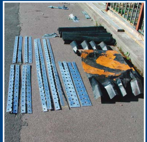
Example of minimal material damage from 113 km/h frontal impact with 1,500 kg vehicle.
