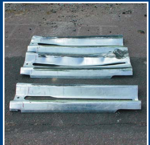
Example of minimal material damage from 114 km/h side impact with a 1,500 kg vehicle.
